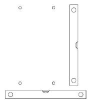
3. Using the drill and 8mm drill bit, drill into the marked positions then insert the wall plugs and tap flush to the finished wall surface.
